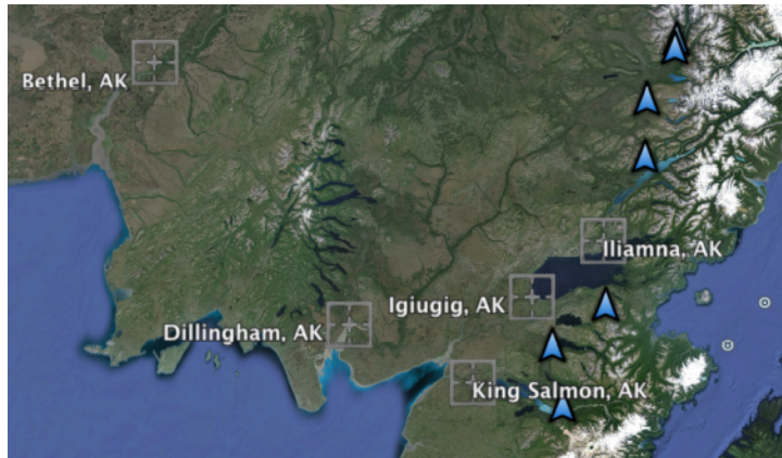
Fig 7. The 7 SWAN monitoring stations provide a north-south transect in Southwest Alaska that complements the Dalton Highway transect. Measurements include soil temperature profiles, snow water equivalent (SWE), precipitation and long-term vegetation study plots [Peter Kirchner, National Park Service].
